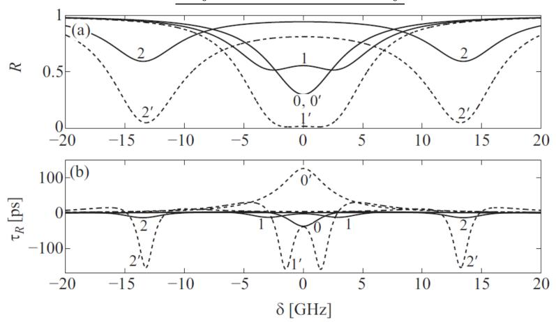
Forward (solid) and backward (dashed) intensity reflection coefficient R and corresponding phase time  $\tau_R$  as functions of detuning  $\delta$ .
