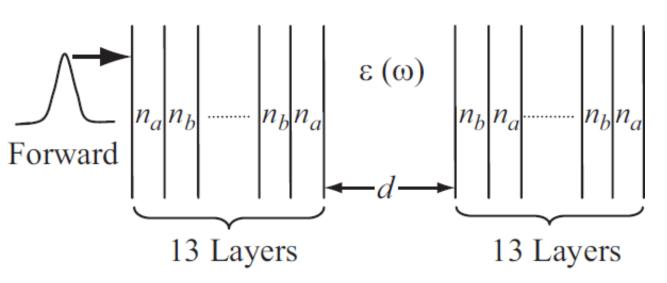
Symmetric FP cavity. The DFB mirrors have 13 alternating high and low index  $(n_a=2.4, n_b=1.3, \text{ respectively}) \lambda/4 \text{ layers.}$
