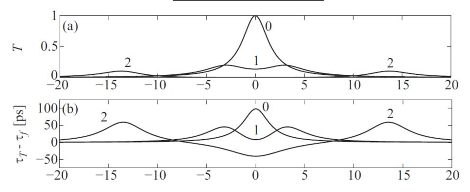
The curves with label 0,1 and 2 are for  $\omega_p^2/\omega_0^2 = 0.0, 0.08 \times 10^{-9}$  and  $1.5 \times 10^{-9}$ , respectively with  $2\gamma/\omega_0 = 1.0 \times 10^{-5}$ .
