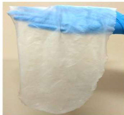
Figure 12: Photograph of proton conducting membrane developed in the laboratory.
