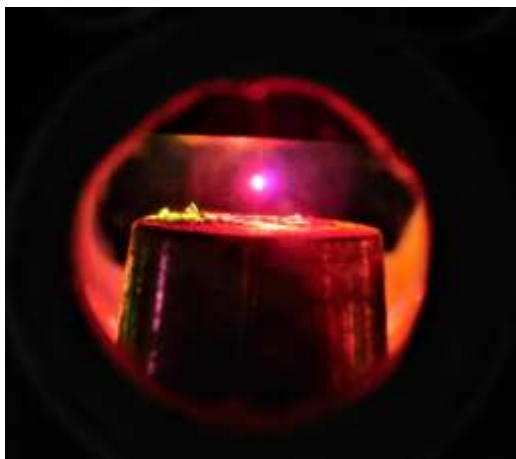
Figure 9: A methanol drop instantly heated to a billion kelvin emits light (visible and x-rays) like the sun.
